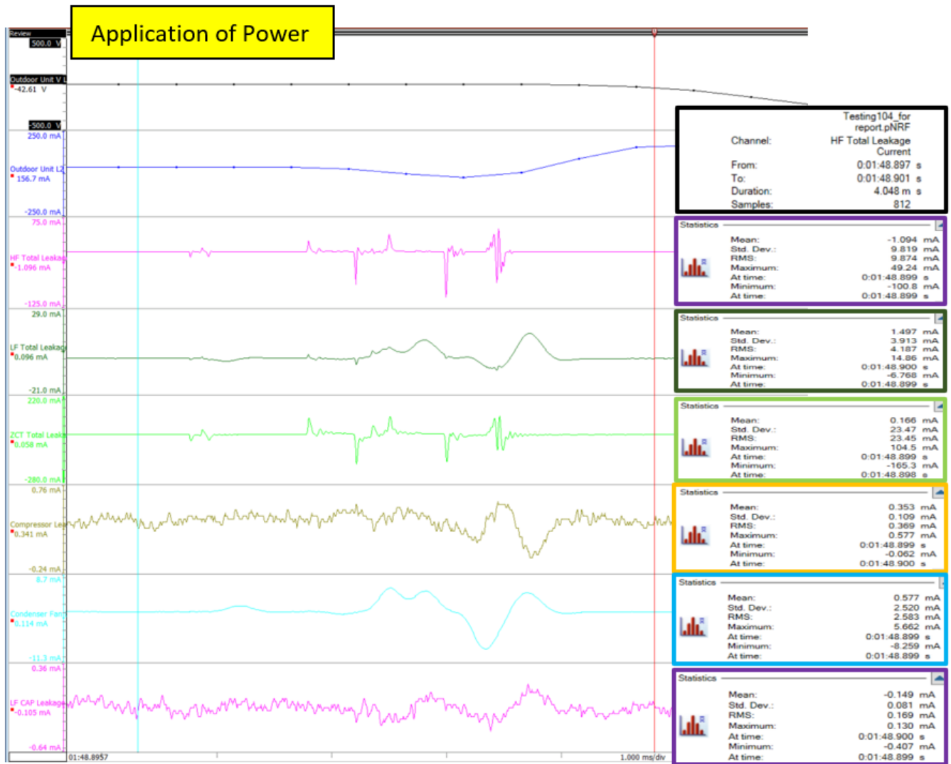
Figure 6-52 Application of Power Leakage Current Waveforms
