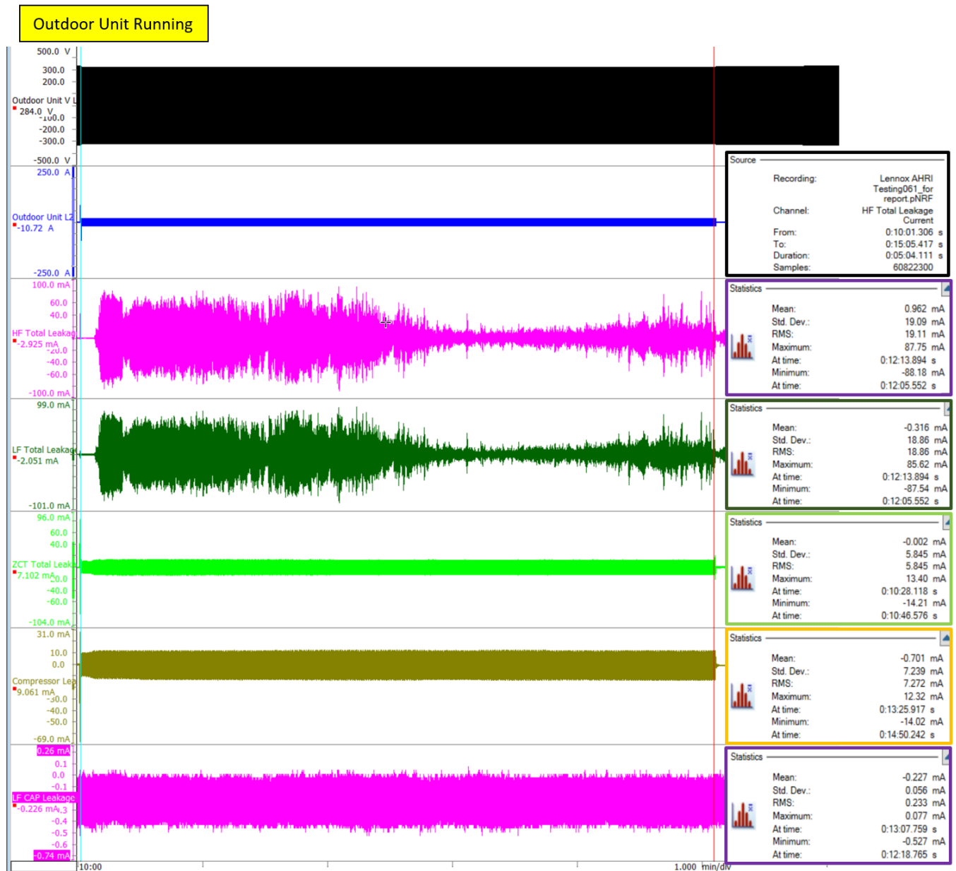
Figure 6-36 Outdoor Unit Running Leakage Current First 20 Minutes
