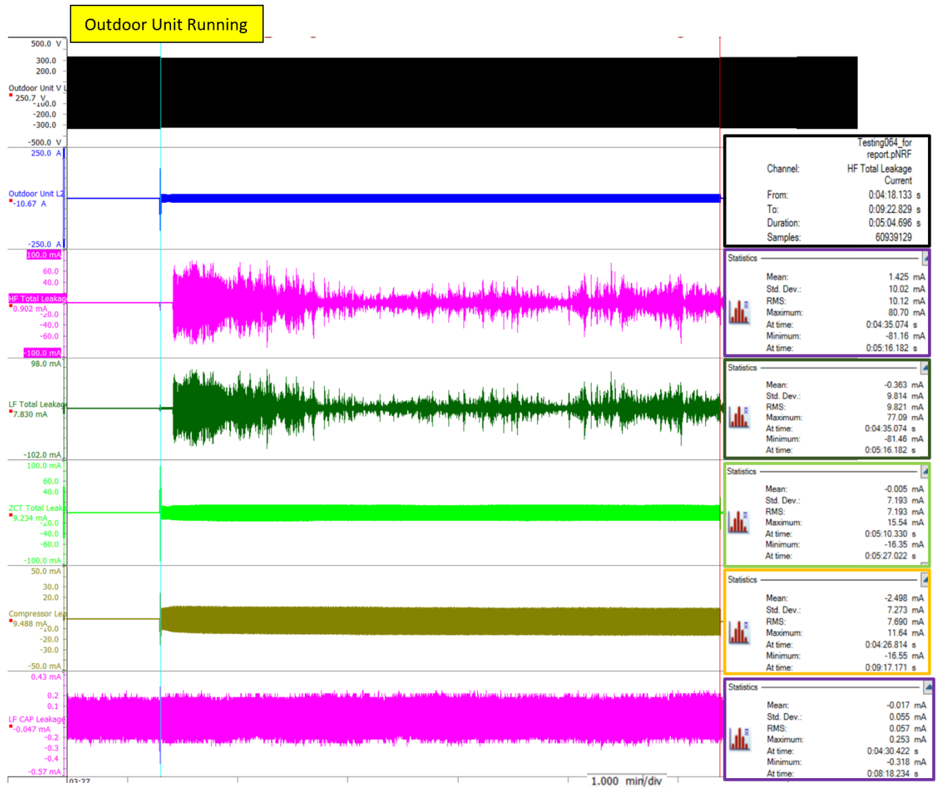
Figure 6-41 Outdoor Unit Running Leakage Current, First 20-Minutes
