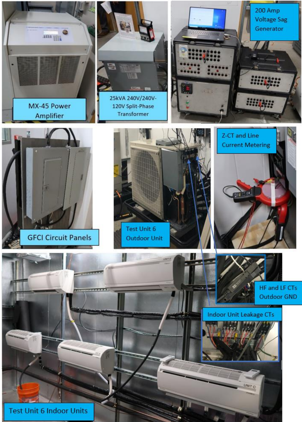
Figure 7-1 AHRI Test Unit 6 Setup
