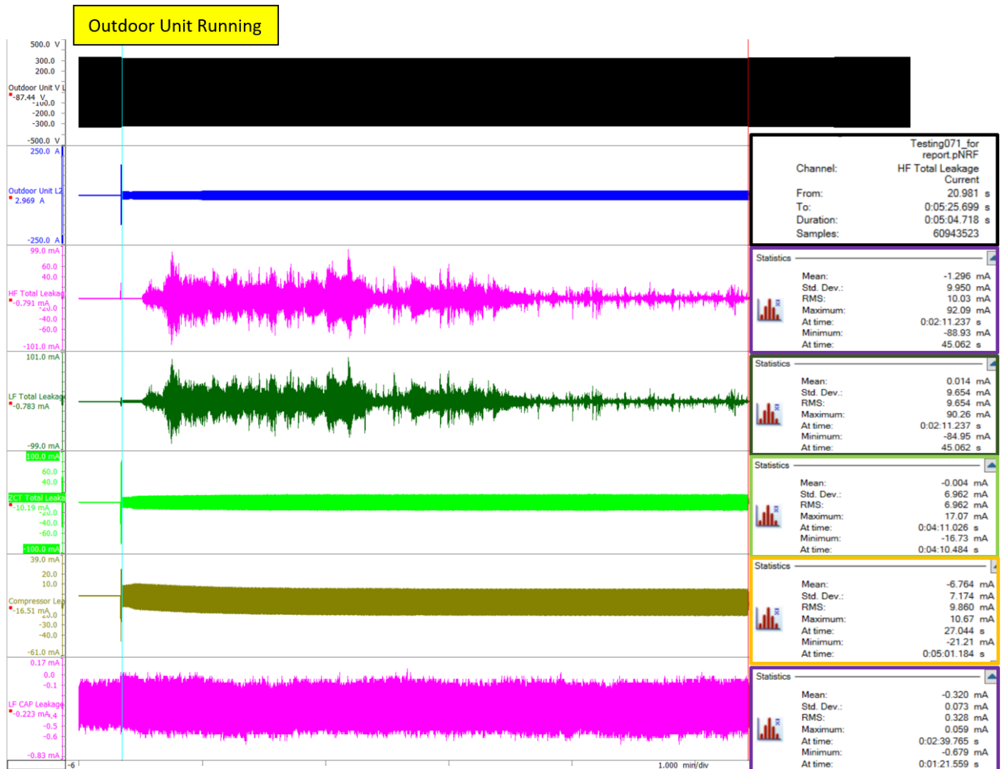
Figure 6-46 Outdoor Unit Running Leakage Current, First 20-Minutes
