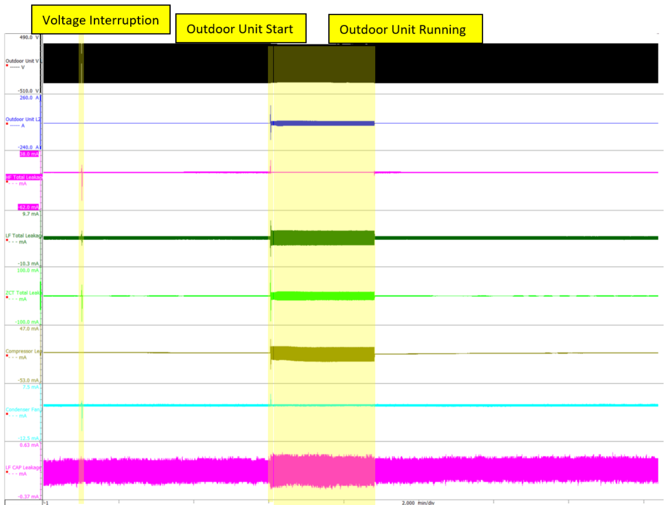
Figure 6-59 Chamber Condition 2, High-impedance Interruption, File 97
