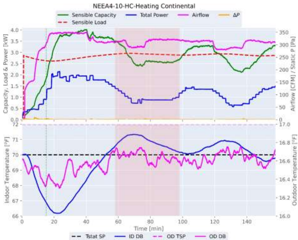
Figure 44. NEEA4-10 (UL) performance and temperature variations for heating continental test interval HC (17°F)
