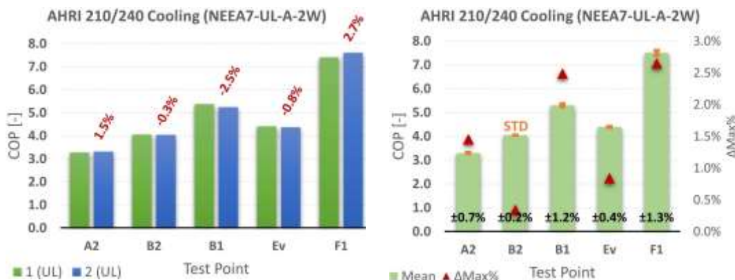
Figure 202. NEEA7 (UL) cooling test results a) COP comparison in different tests b) Test intervals mean COP with STD and maximum difference among repeated tests
