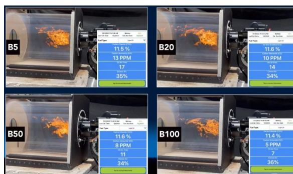
Figure 36: Burner Operating with B5 through B100 Low-Carbon Liquid Fuels (Source: NORA)
