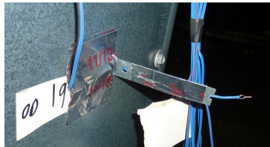
Figure C11. Typical Thermocouple Temperature Measuring Device Mounting
