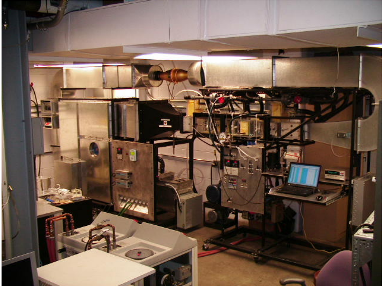
Figure 9 The third generation wind tunnel. The air handler lies on the left half of the photo, while the test section and instrumentation is on the right half.
