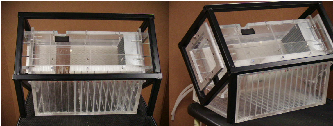
Figure 44 Final test section design. Note the section of honecomb material removed and the addition of a drift eliminator at the exit of the test section (air flows from left to right).
