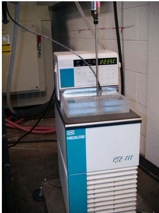
Figure C1 Calibration of Thermistors using Kaye Intelligent RTD Temperature Probe.
