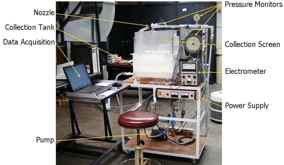
Figure 7 Photograph of the experimental system arrangement.
