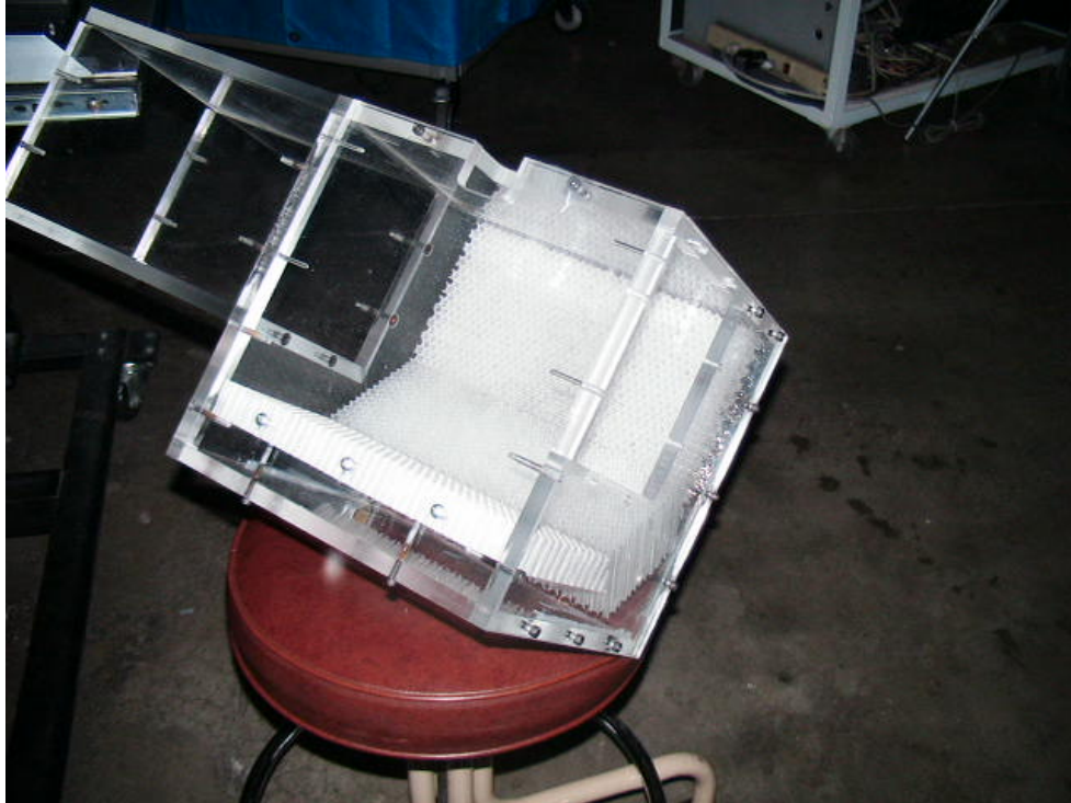
Figure 47 Test section incorporating the lowered wall concept with the three piece wall design.
