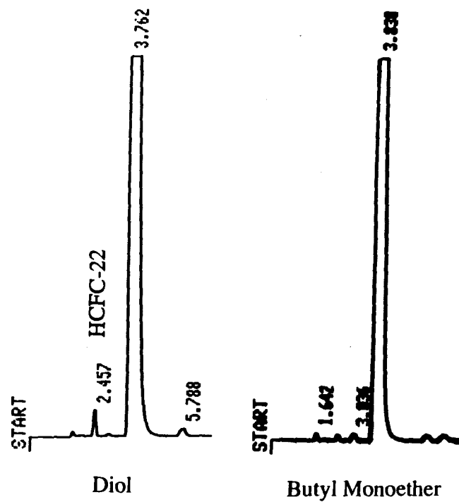
Figure A-9. Gas Chromatograms of CFC-12/Polypropylene Glycol Mixtures Aged at 175°C (347°F) for One Week in the Absence of Valve Steel Catalysts. In Situ Conductivity Test Method.
