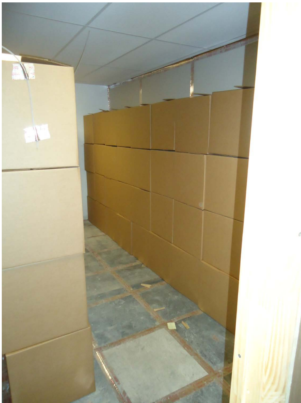
Figure 3.21 Example of Obstructions Simulated with Cardboard Boxes (Restaurant Scenario, Walk-in Interior)
