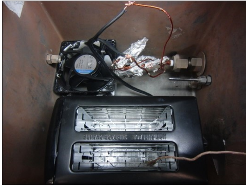
Figure 16.1. Toaster installed in the test chamber (Proctor, Silex, $9.99).
