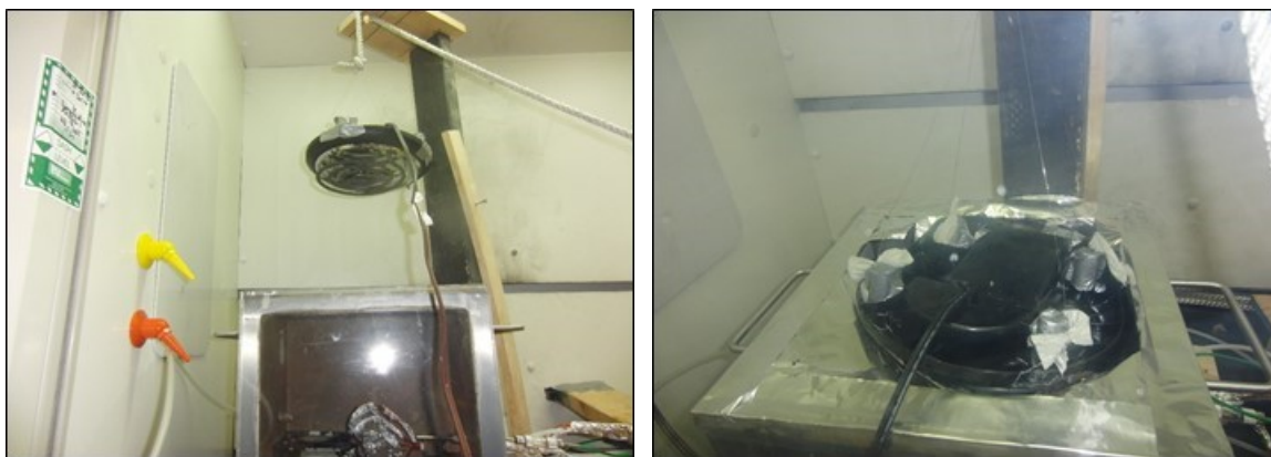
Figure 17.1. Images of the hot plate insertion tests. The hot plate excitation was 750 W and 120 VAC (Kitchen Selectives, $11).
