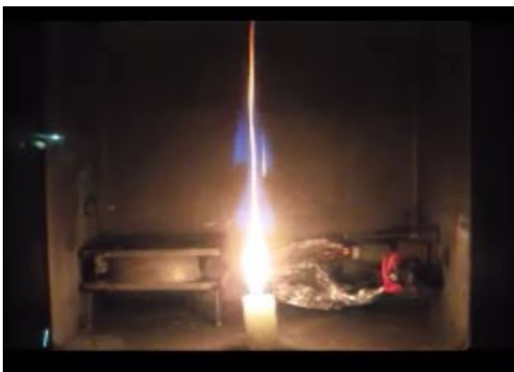
Figure 7.5. Lower leak with approximately 3% R-1234yf.
