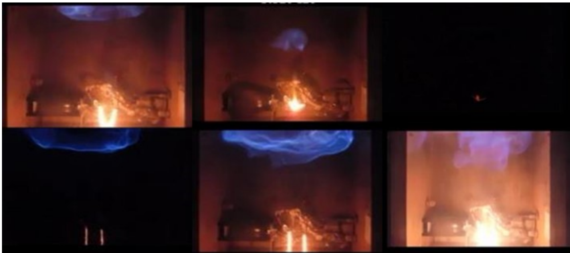
Figure 4.6. Hot wire in R-1234ze (Premixed): 6.5% (LFL = 6.5%).
