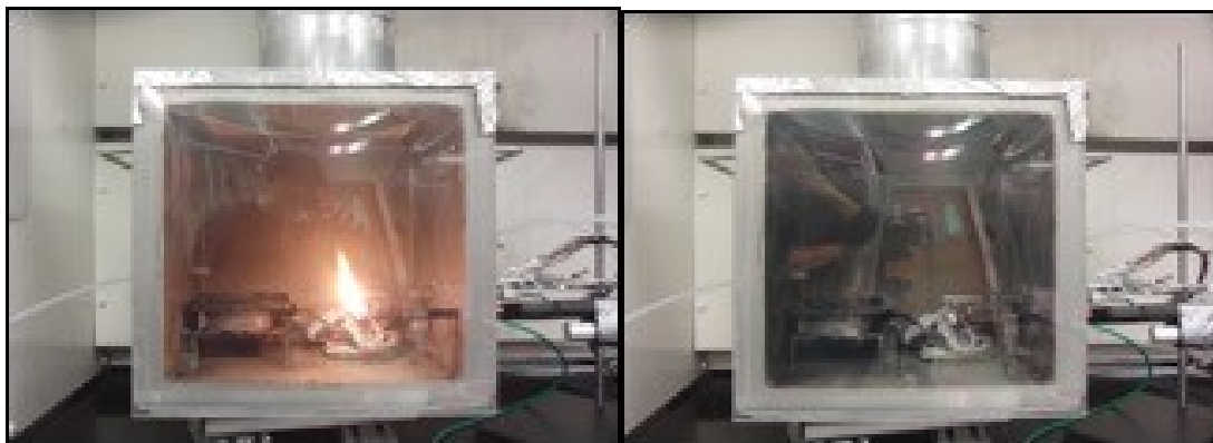
Figure 9.2. Barbeque lighter (second method) testing, with 2% R-32 (left) and 3% R-32 (right).
