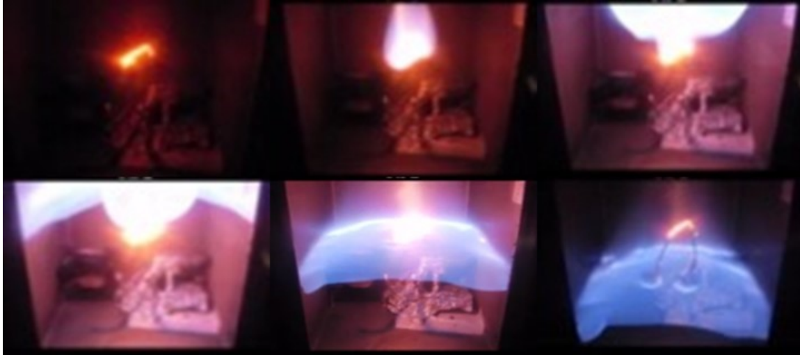
Figure 4.3. Hot wire in R-32 (premixed), 17% (LFL=14.4%).
