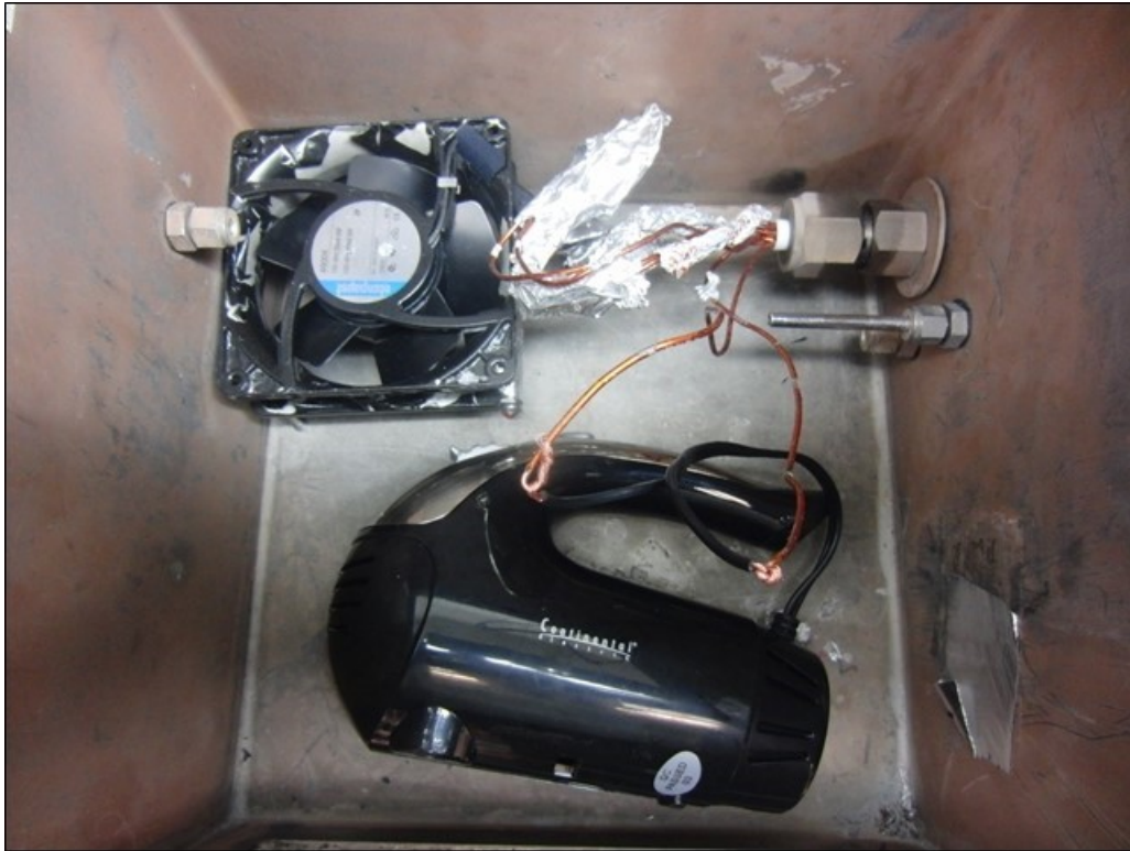
Figure 12.1. Test chamber interior with mixer installed.
