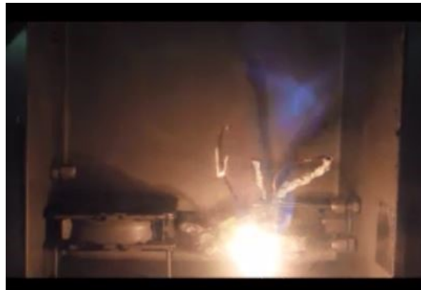
Figure 4.4. Hot wire in R-32. The flammability limit is estimated at 11.5% concentration of R-32.
