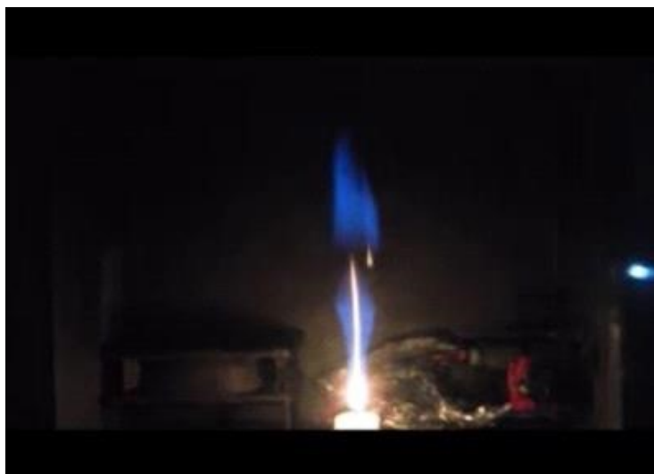
Figure 7.4. Upper leak with approximately 4% R-1234yf.
