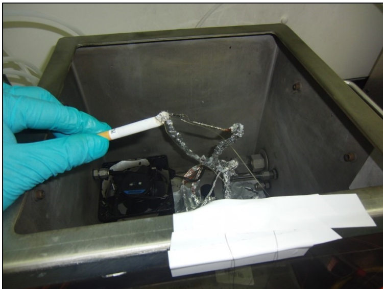
Figure 8.1. Cigarette temperature measured by a bare thermocouple in air.
