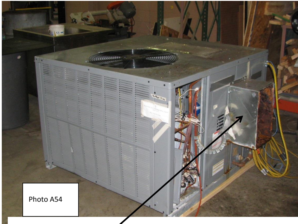
Artificial Collector Box Placed Around Standard Vent Discharge to Capture Flue Products and Discharge Outdoors
