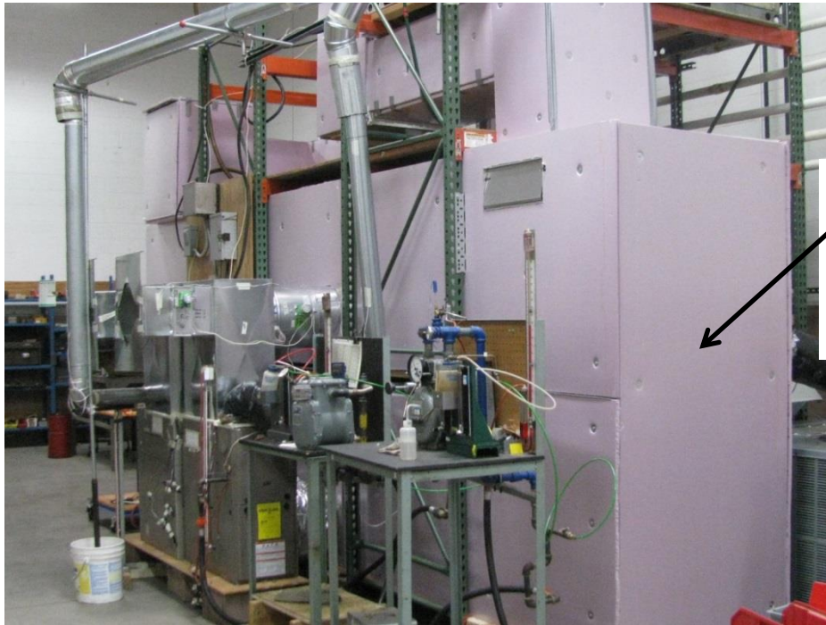
Layout of the Air Cooling System for Low Inlet Air Temperature Study
