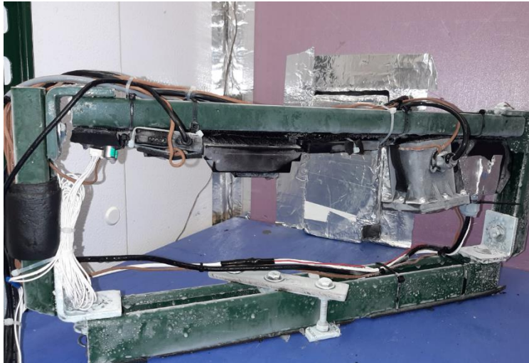
Figure 3-40. Tested Sensors towards the End of the Condensation Test
