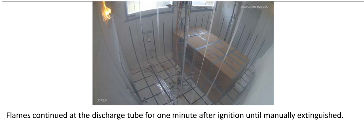
Figure 211 – CP_21: Continued flaming from expanding propane in the discharge tube
