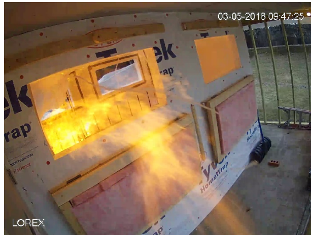
Figure 152 – CP_12 Flame extension through the west side vent
