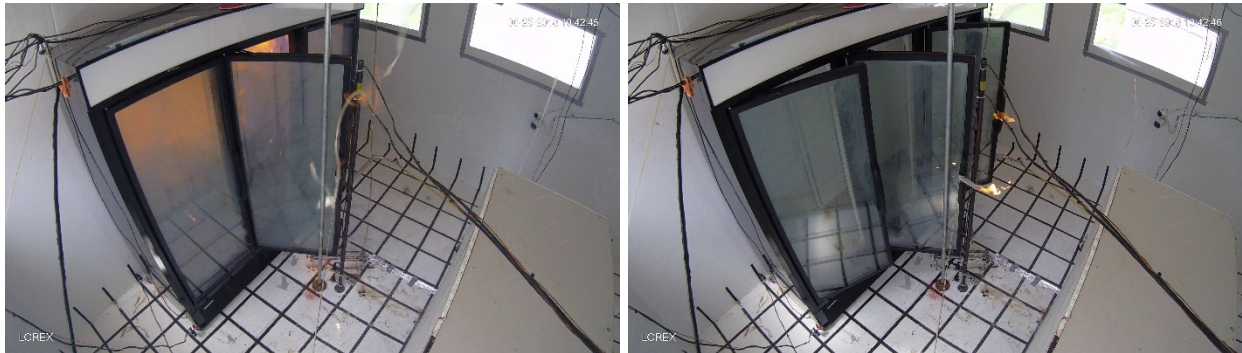
Figure 442 – RI_12 Deflagration showing doors forced open due to developed pressure.
