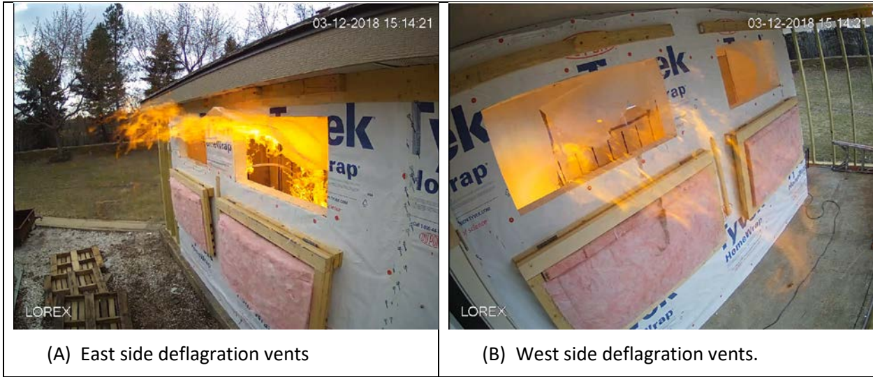
Figure 234 – CP_25 Deflagration Vents Bursting with Flame Extension
