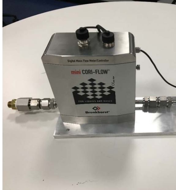
Figure 6 – Mass Flow Meter
