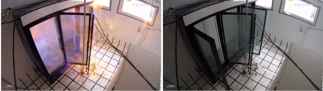
Figure 428 – RI_10 Deflagration showing doors forced open due to developed pressure.
