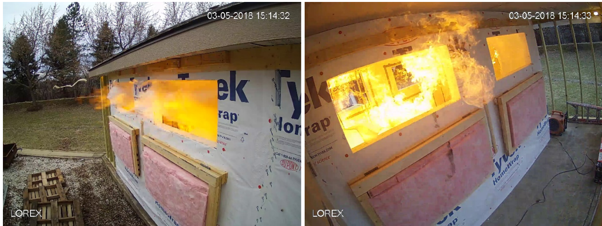
Figure 186 – CP_17 Flame extension through the west and east side vents
