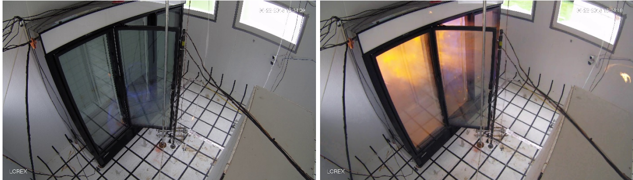
Figure 435 – RI_11 Deflagration showing initial pre-mixed flame (left) and small deflagration (right)
