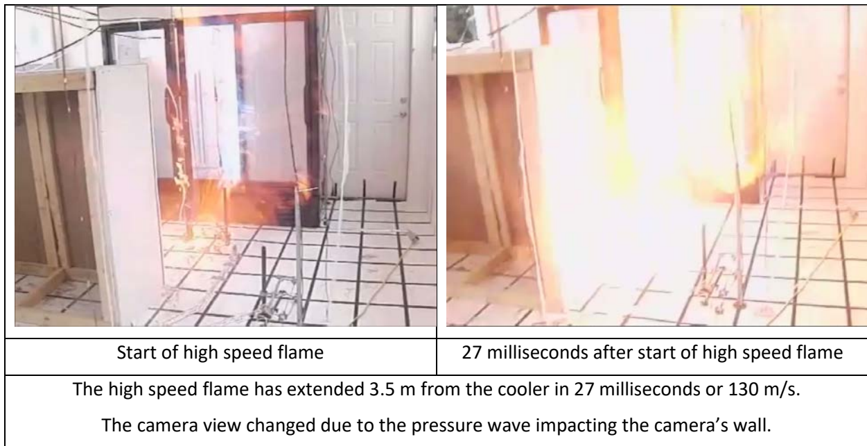
Figure 478 – RI_18 Deflagration Overpressure Effects
