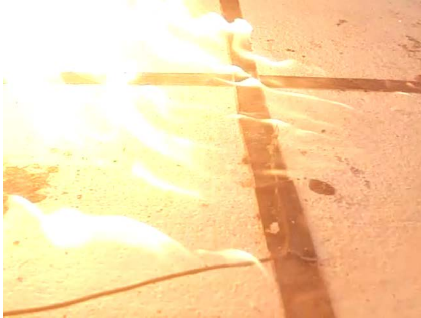
Figure 42 - PTAC_17 (217 g; Fan On). Flames attached to a pool of liquid propane
