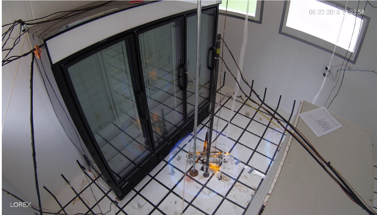
Figure 488 – RI_20 Simultaneous Ignition at Locations A and B
