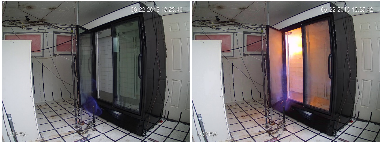
Figure 415 – RI_08 Ignition (left) and small fireball (right).
