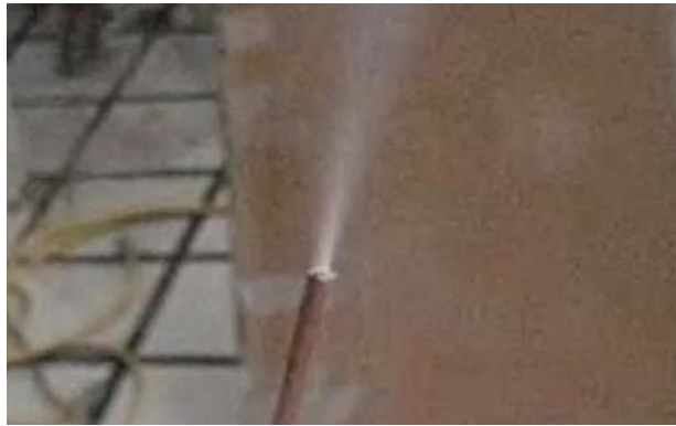
Figure 59 – Capillary Tube showing liquid mist at the exit
