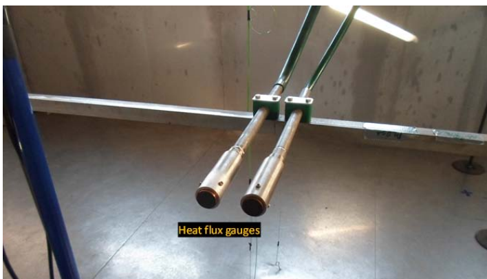
Figure 5.4: Heat flux gauges - one with a high range and fast response time and one with a lower range and slower response time.
