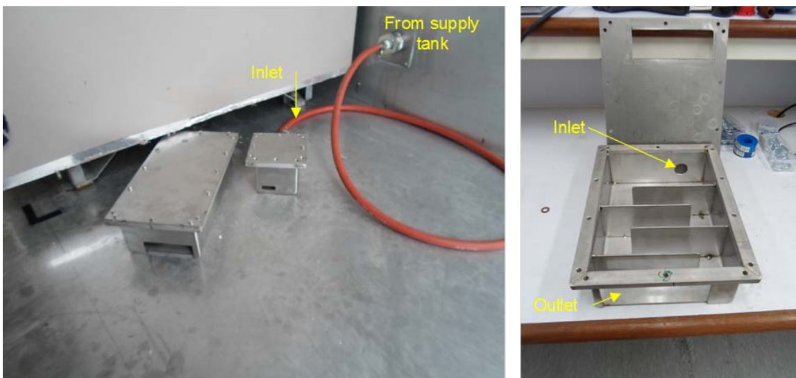
Figure 4.4: Release boxes used to create highly impinged low-momentum releases.
