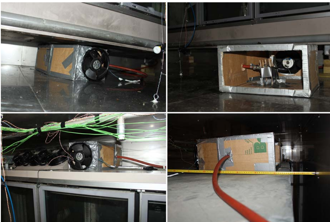
Figure 4.6: Mock-up condensing unit to replicate releases with the condensing fan on.
