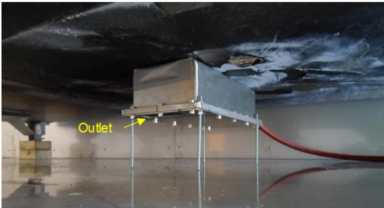
Figure 4.5: Leak box positioned below the display case.
