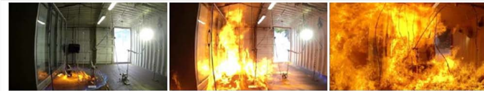
Figure 5.41: R-454C vs R-290 test comparison #5.
