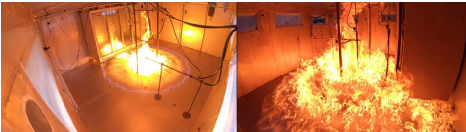
Figure 5.37: R-454C vs R-290 test comparison #1.
