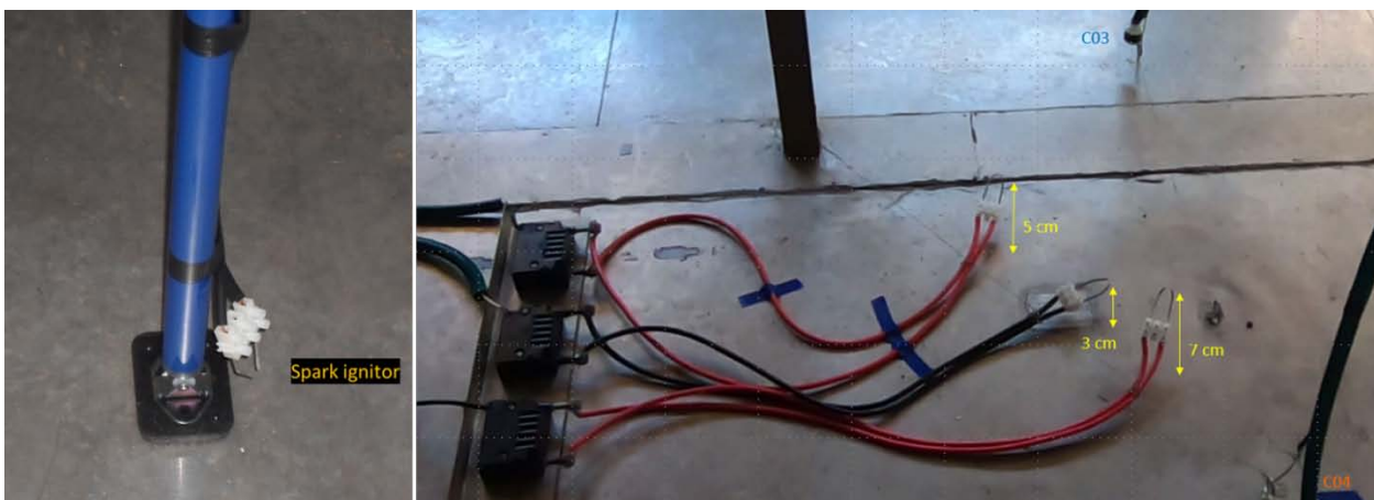
Figure 5.5: Spark ignitor setup during external R-290 release tests (left image) and external R-454C release tests (right image).
