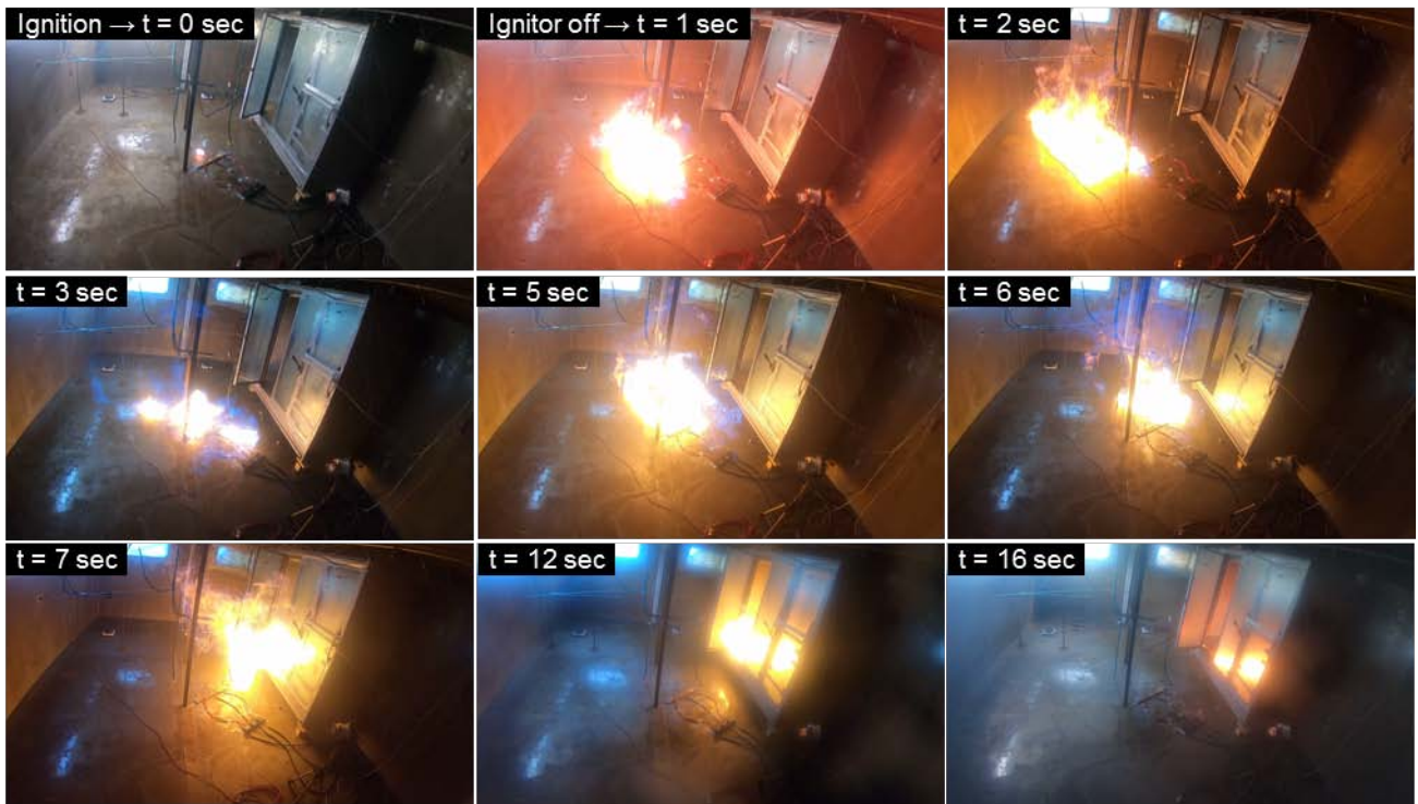
Figure 5.32: Test #19 flame evolution after ignition.
