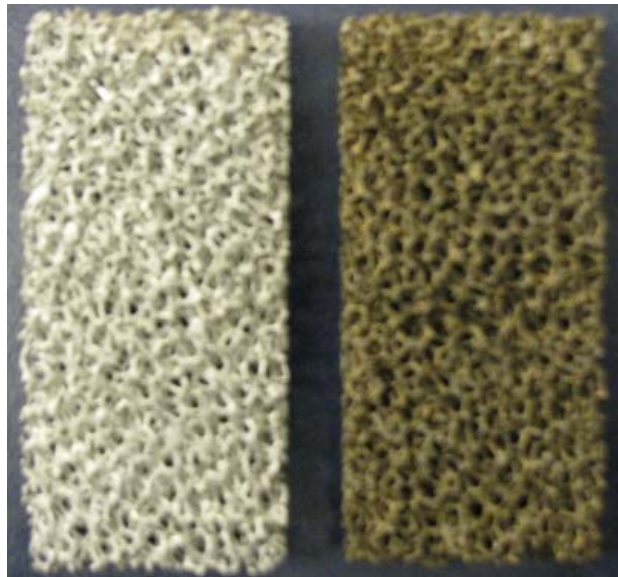
Figure 1.18: 10 PPI Metal foam sample before and after treatment
