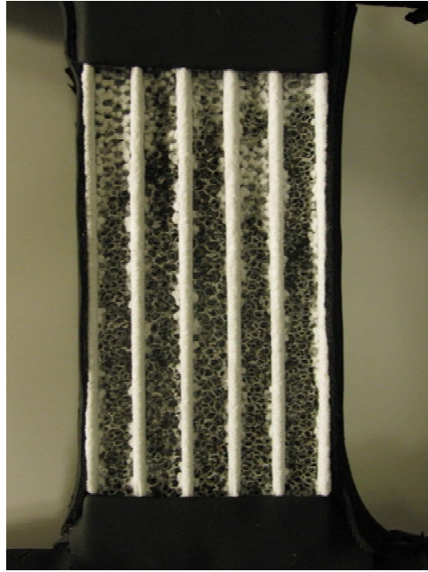
Figure 2.6: Frost formation for 10 PPI foam
