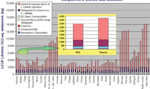
Figure 1: LCCP CO<sub>2</sub>-eq. Direct and Indirect contributions of baseline R134a system (Papasavva et al., 2010)
