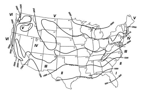
Figure 8: Heating Load Hours (HLH<sub>A</sub>) for the United States
