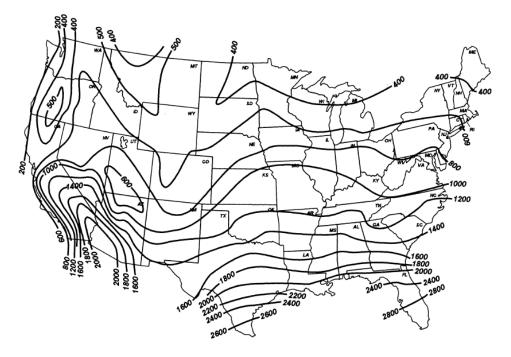
Figure 7: Cooling load hours (CLH<sub>A</sub>) for the United States
