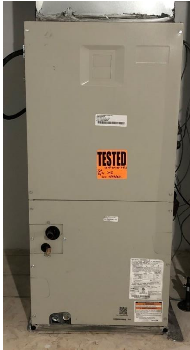
Air Handler for Horizontal and Vertical Tests: Nortek Model B6VMMX24K-B
