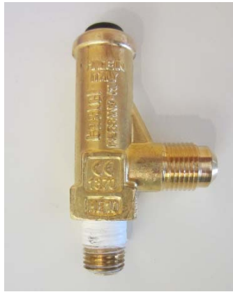
Figure 4.36: Pressure relief valve n°2.
