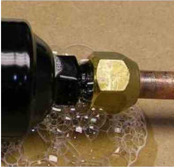
Figure 2.30: Leaks at flare fittings.
