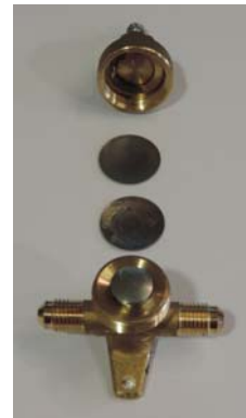
Figure 4.26: Expanded view of manual valve n°2.
