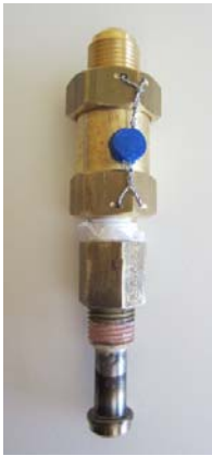
Figure 4.35: Photo of prepared pressure relief valve n°1.
