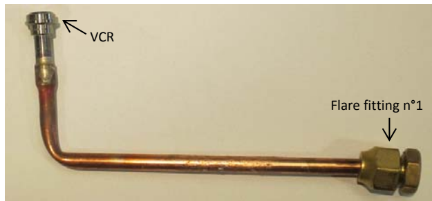
Figure 4.13: Preparation of flare fitting n°1.
