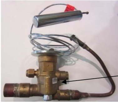
Figure 4.27: Photo of prepared TXV n°1.
