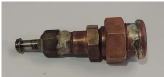
Figure 4.54: Prepared service valve n°1.
