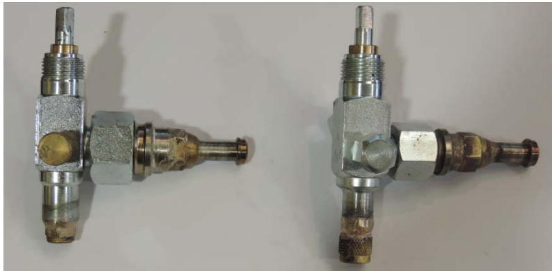
Figure 4.52: Prepared service valves n°3 and n°4.
