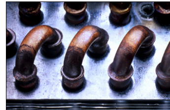
Figure 2.34: Brazed joint of coil
