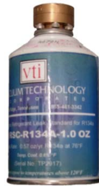
Figure 3.4: HFC-134a calibrated leak.
