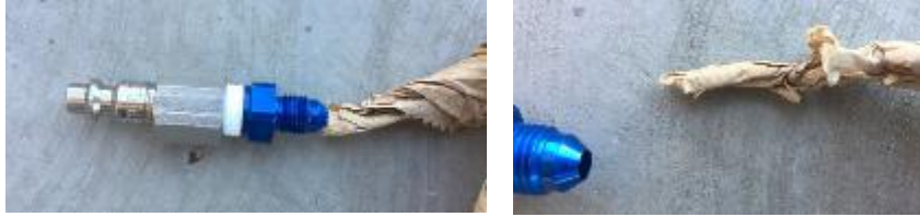
Figure 10 Test to verify that applying a vacuum to the cylinder did not pull POE oil out of the cylinder.
