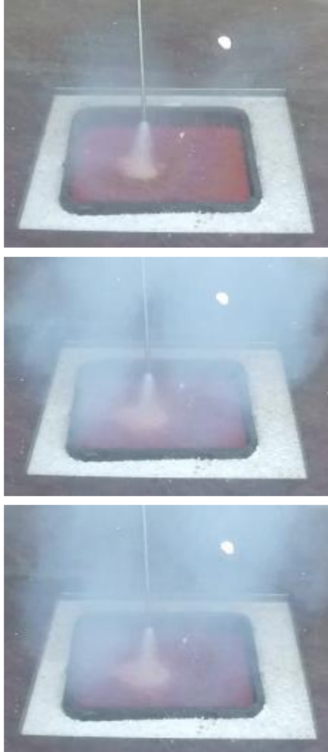
Figure 14 Screenshots of ejection in 3/120s increments for test ID36 with R452B refrigerant mixed with 3% POE oil by mass, and with a hot plate temperature of 800°C (1472°F).
