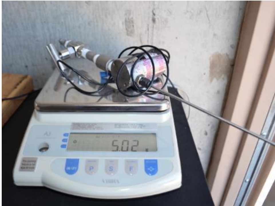
Figure 9 Refrigerant charge assembly. Note that the weight of the assembly has been tared, and the scale display is showing the charge of refrigerant in the chamber.
